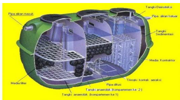
Gambar Detail Biofilter
