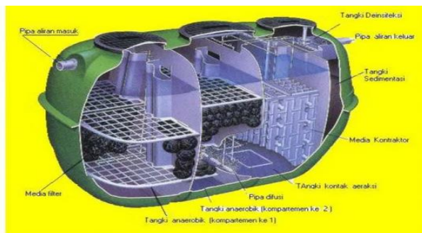
Gambar Detail Biofilter
